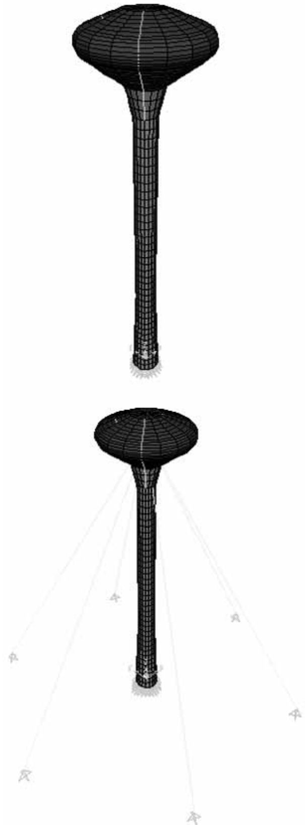
Slika 2. Modeli vodotornja bez zatega – gore i sa zategama – dolje Figure 2. Models of the liquid storage tank without ties – up and with ties – down
